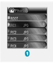
Select **Photo** on the main menu and press M to enter the ROOT folder with listed photos under it. You can select different photos by pressing < / >, and press  $\gg$  to view.
